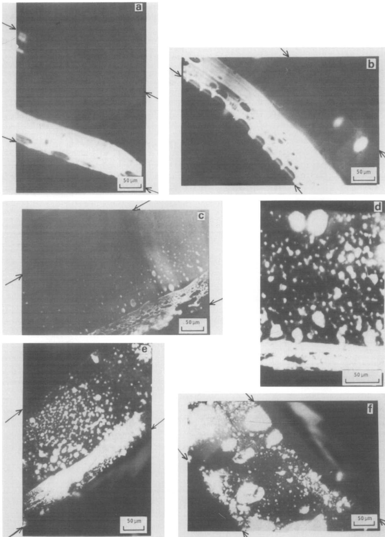
**Figure 1** Optical micrographs of cross sections of PMMA/polycarbonate blends (65/35 w/w) cast under varying conditions (see Table 1). Arrows indicate the edges of the films. Scale bars represent 50  $\mu\text{m}$
