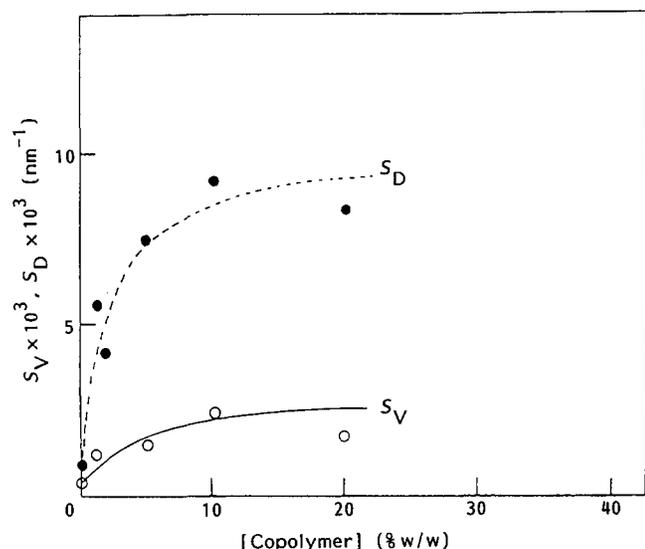
**Figure 7** Effect of copolymer concentration (% w/w) on the interfacial area per unit total volume,  $S_V$  (○) and per unit volume of dispersed phase,  $S_D$  (●)
