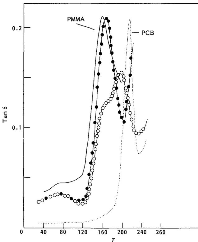
Figure 11 Dynamic mechanical spectra of PMMA (—), polycarbonate homopolymer (.....), PMMA/polycarbonate blend (65/35 w/w) (O) and the same system with 20% w/w added copolymer (●), using supported specimens
