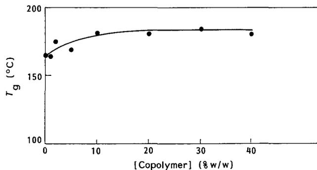
Figure 10 Variation of  $T_g(\tan \delta)_{\max}$  of PMMA/polycarbonate blends (65/35 w/w) with added copolymer concentration
