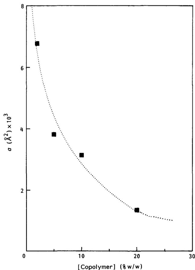
**Figure 8** Variation of area occupied by a single copolymer at the interphase with added copolymer concentration as calculated by equation (3)
