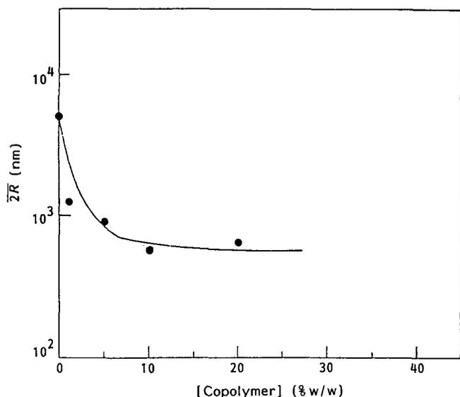
**Figure 5** Variation of the average diameter of polycarbonate-rich domains with varying added copolymer content in PMMA/polycarbonate (65/35 w/w) blends
