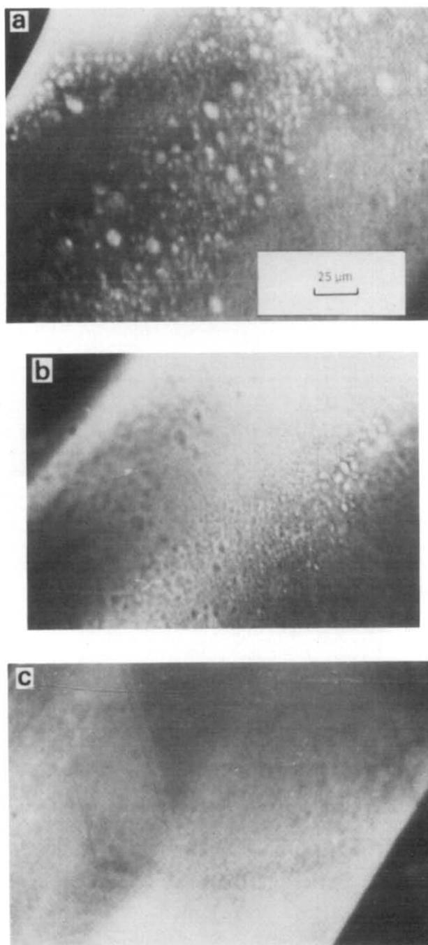
**Figure 3** Optical micrographs of cross sections of PMMA/polycarbonate blends (65/35 w/w) containing (a) 2, (b) 5 and (c) 10% w/w copolymer
