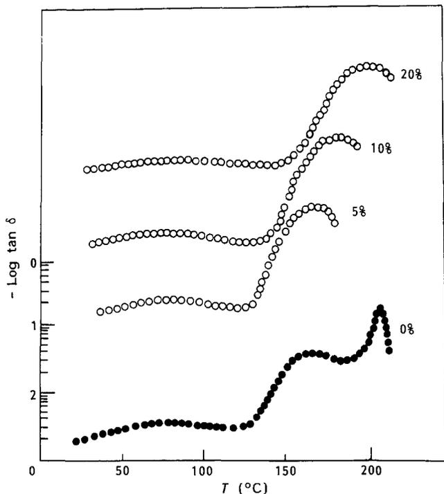
Figure 9 Logarithmic decrement curves for PMMA/polycarbonate blends (65/35 w/w) containing 0, 5, 10 and 20% w/w added copolymer
