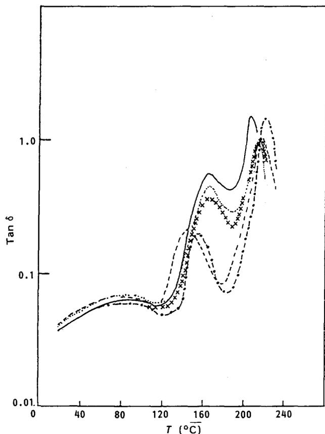
**Figure 2** Effect of film casting procedure on dynamic mechanical properties of 65/35 w/w PMMA/polycarbonate blends: —, sample A; - - -, sample B; x x x x, sample C; . . . ., sample D; — — —, sample E. Casting procedures are given in Table 1
