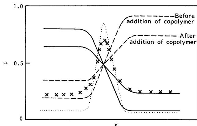
**Figure 14** Density profile of PMMA/polycarbonate blend (65/35 w/w): —, PMMA-rich phase; - - -, polycarbonate-rich phase; ····, copolymer at low copolymer contents in the blend (<5% w/w); × × × ×, copolymer at higher copolymer contents in the blend (>5% w/w)
