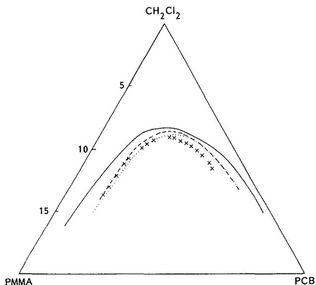
Figure 12 Effect of added copolymer concentration on the experimentally determined phase diagram of PMMA/polycarbonate blends (65/35 w/w): —, 0%; x x x, 13%; - - -, 9%; . . . ., 4.8%
