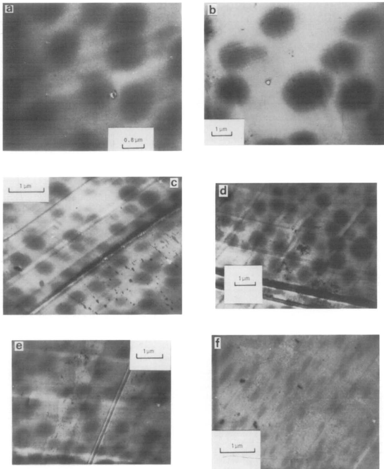
**Figure 4** Transmission electron micrographs of PMMA/polycarbonate blends (65/35 w/w) containing (a) 1, (b) 2, (c) 5, (d) 10, (e) 20 and (f) 30% w/w copolymer
