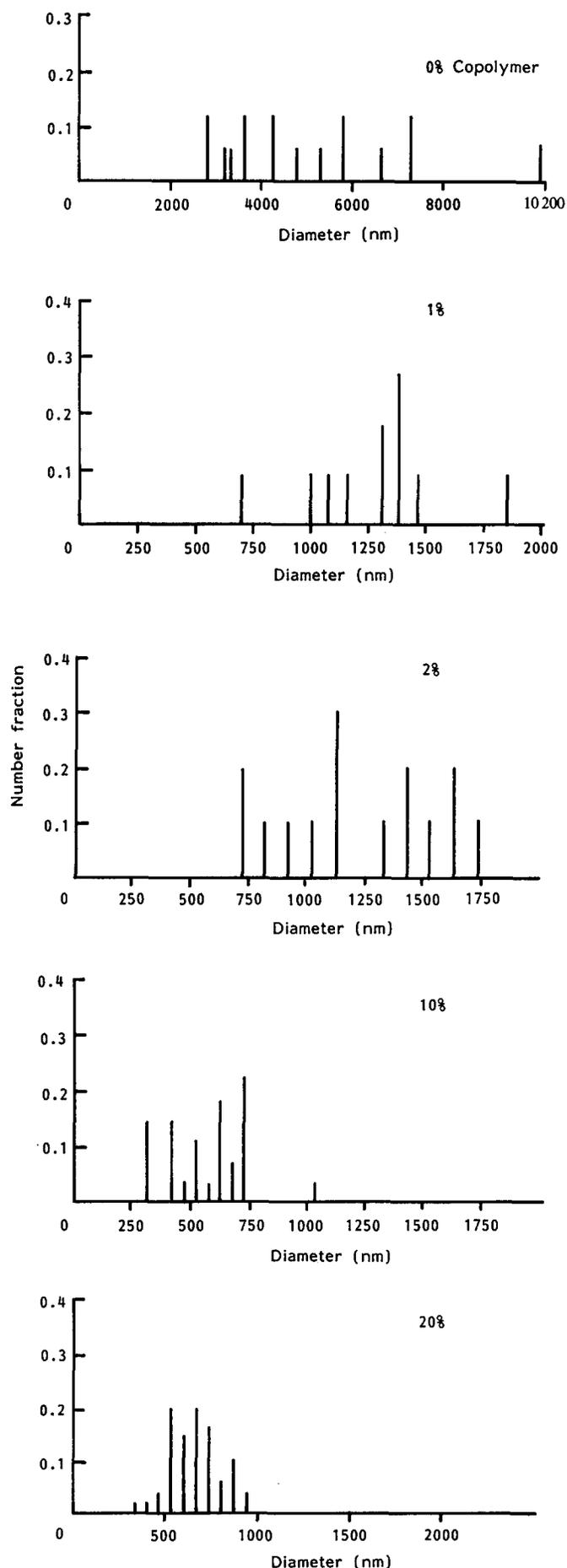
**Figure 6** Histograms of the relative frequency of polycarbonate-rich domain diameter for PMMA/polycarbonate blends (65/35 w/w) with varying copolymer content
